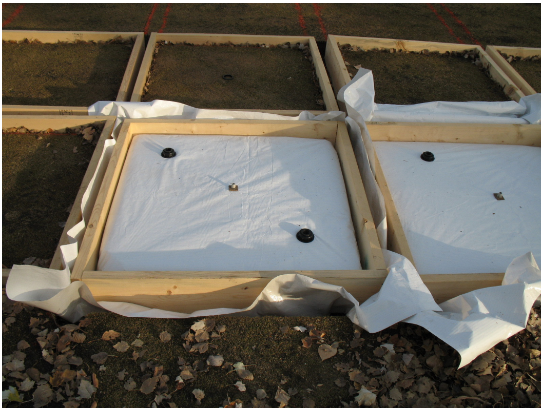
Figure 1. Trial in Olds showing impermeable cover prior to ice development
